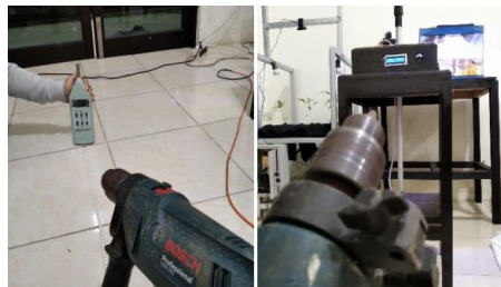
Figure 12. Tests on SLM and sensors
