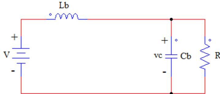
Figure 3. The boost converter circuit when the transistor is Off.
