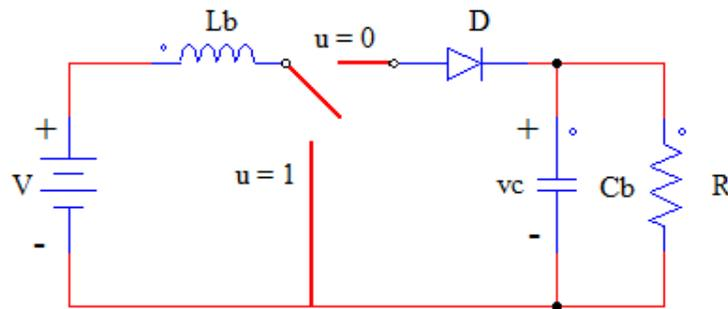
Figure 4. The boost converter circuit with an ideal switch.
