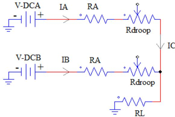
Figure 5. Boost converter connected in parallel with different output voltages.
