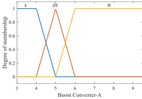
Figure 7. Membership function of boost converter-A.
