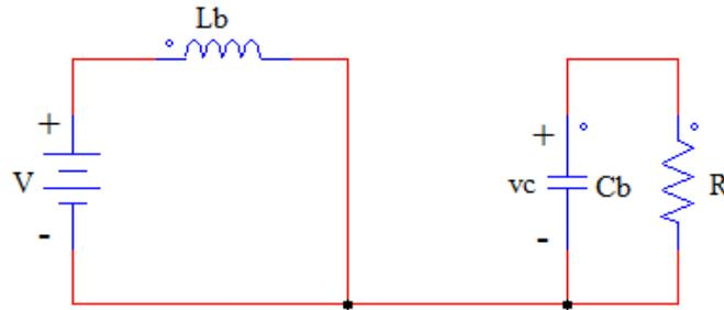
Figure 2. The boost converter circuit when the transistor is On.
