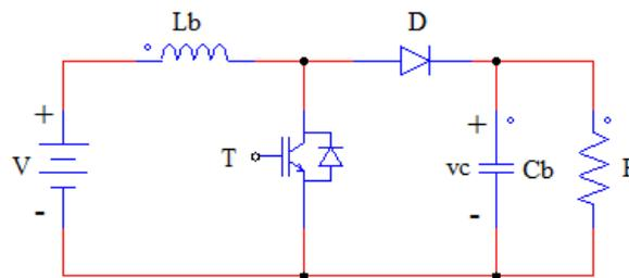
Figure 1. Basic boost converter circuit.
