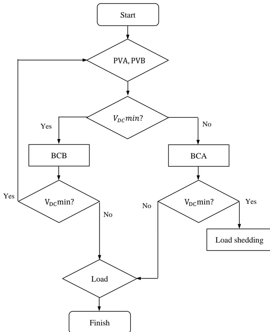
Figure 11. Flowchart boost converter connected in parallel.
