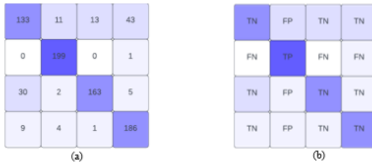
Figure 5. Confusion matrix table with 10 epochs experiment: (a) Confusion matrix results, (b) Original label and prediction results
