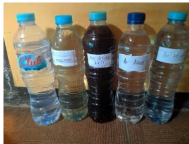
Figure 1. Sample water type for TDS sensor testing
