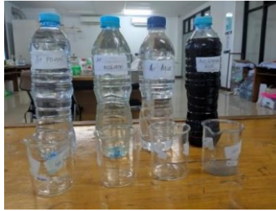
Figure 3. Type of water sample for turbidity sensor testing
