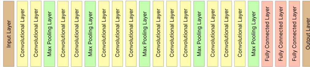
Figure 4. The architecture of VGG16
