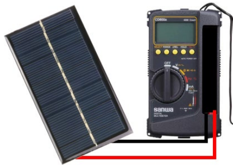
Figure 5. Schematic of Voltage Measurement at Solar Panel Output
